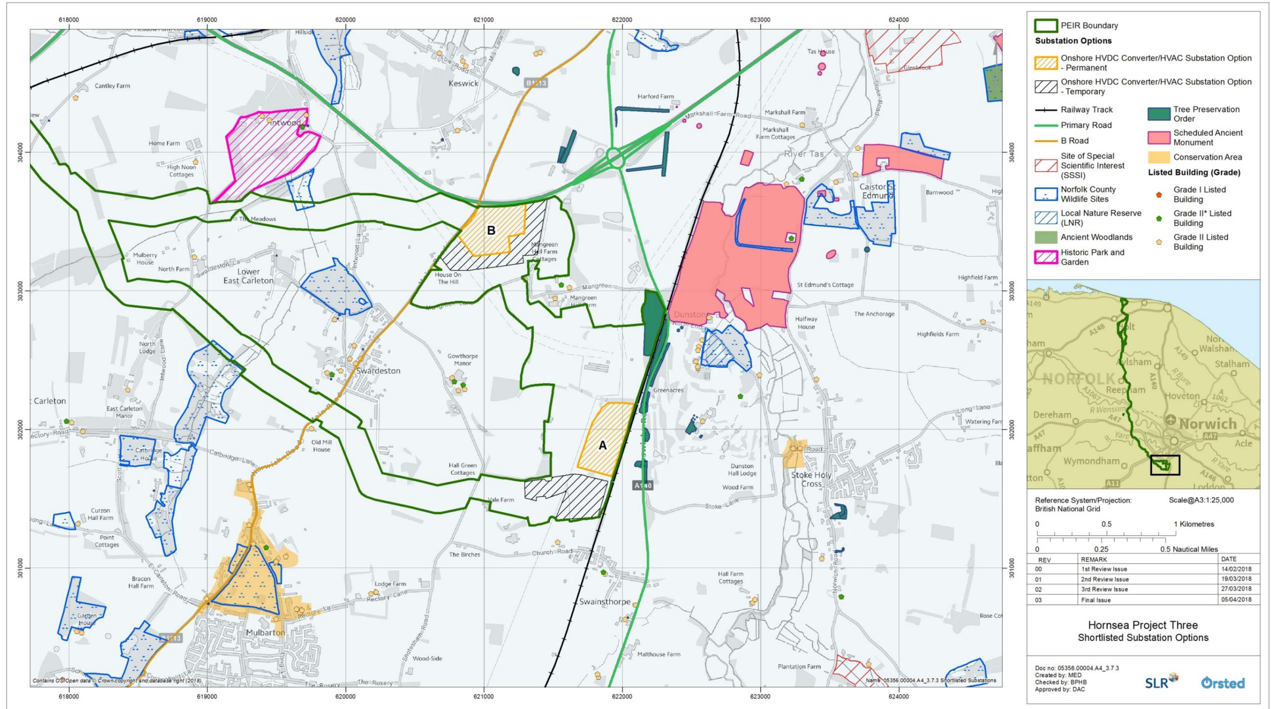
Figure 3.8: Shortlisted Substation Options.
